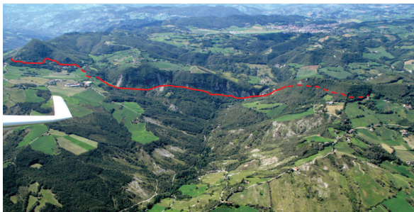
Fig. 12 - Air view of the geologic contact (red line) between the Arenarie di Bismantova and the underlying shaly Ligurian Units. The Lerna Stream headward erosion (see text) is evidenced.
