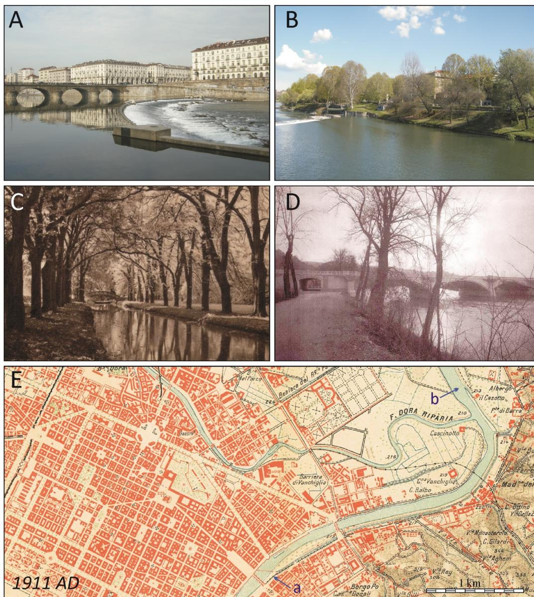
Fig. 14 - Weir near the Vittorio Emanuele 1st Bridge (A) and entrance of the Michelotti Canal (B) in the right bank of the Po River; (C) ancient photograph (1884) of the Michelotti Canal, crossed by the Eiffel iron bridge; (D) arch preserved in the Sassi Bridge on the Po R. for the canal flow; (E) ancient topographic map (IGM, 1911) that reports the Michelotti Canal on the right of the Po R., from the weir (a) to the return to the stream (b).
