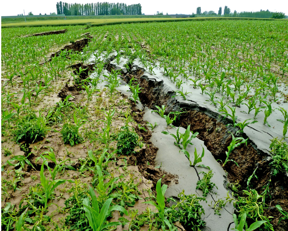
Fig. 19 - San Carlo. Coseismic surficial breaks associated to liquefaction (linear ejection of sand and water). Note the echelon geometry of fractures that mimic a graben-like feature (i.e., lateral spreading of the paleo-Reno River ridge). Buildings, roads, walls and pipelines located above this fractures have been seriously damaged the night of May 20.
