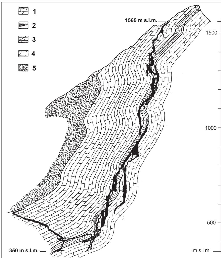
Fig. 4 - Sketch geologic profile of Olivifer Cave: note the structure-controlled vertical pattern of the cave. 1) Dolomitic marble, 2) phyllite lens, 3) shaly marble, 4) dolomite, 5) Palaeozoic basement. (from: Piccini, 1992).
