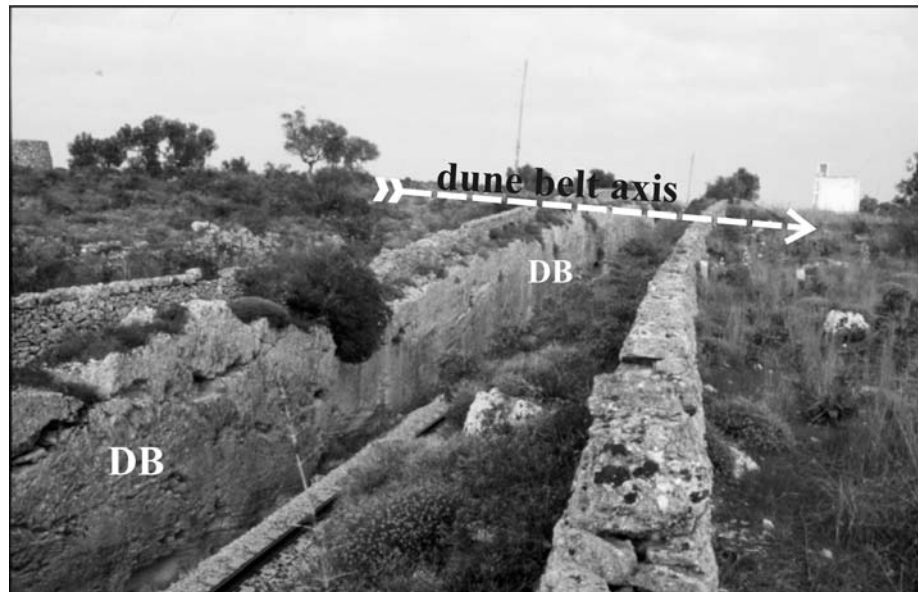
Fig. 7 - Outcrop of sandy dune belt (DB) some meters thick in a railway cutting in the hinterland of Gallipoli. The photo shows also the classic curve shape of the dune belt with the axis elongated perpendicularly to the cutting.
