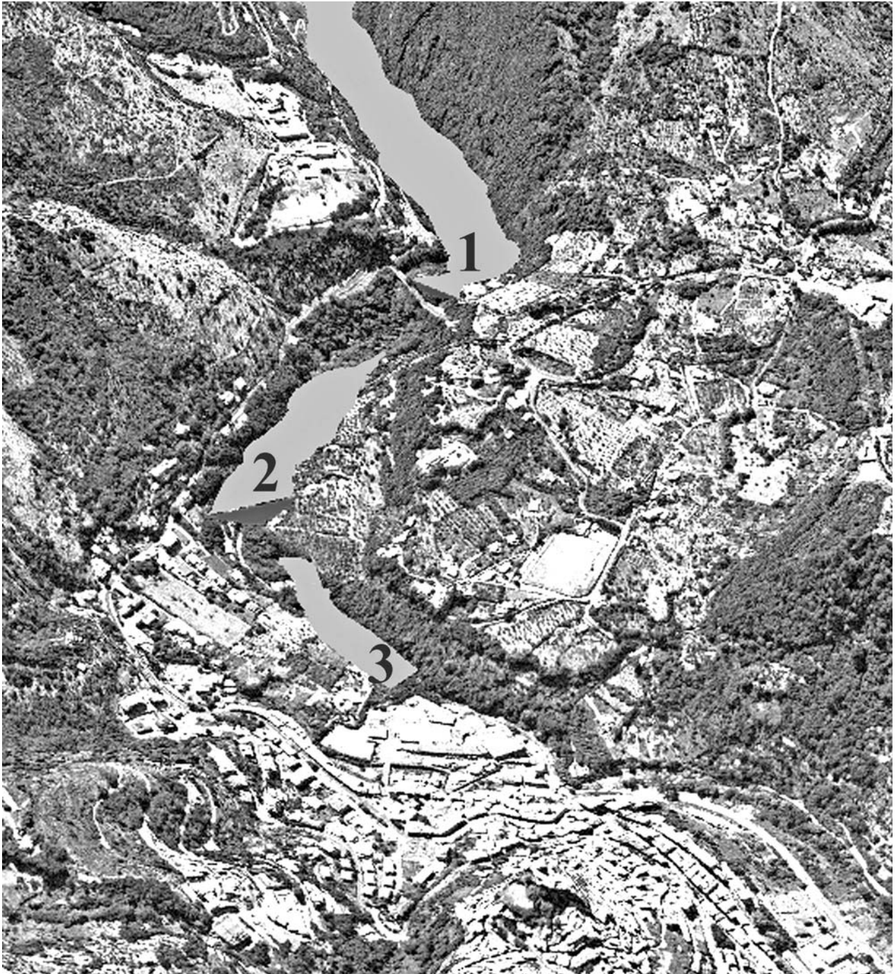
Fig. 21 - Hypothetical reconstruction of the lakes in the Subiaco area, formed by the Neronian dams at Ponte S. Mauro (1) and Parata (2) and by the dam of XV century at Cartiera di Subiaco (3).
