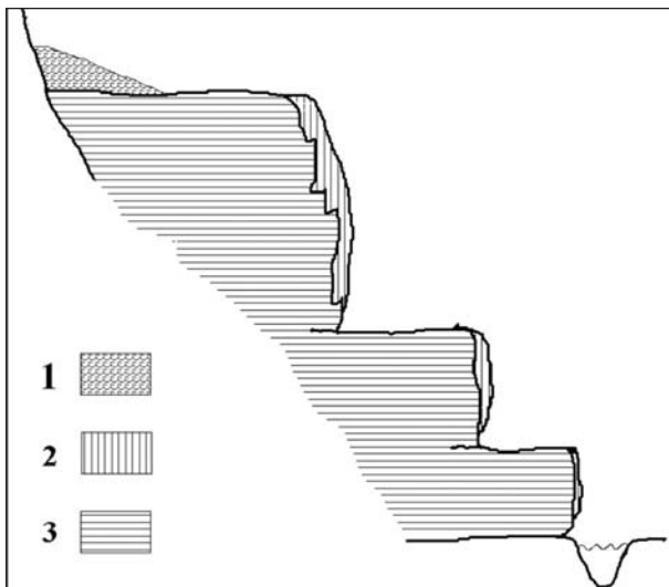
Fig. 6 - Profile sketch (not to scale) of the three depositional terraces of Fig. 5. Legend of symbols: 1 Pedogenized soil colluvium rich in volcanic minerals; 2 Cascade moss phytohermal lithofacies; 3 Mainly microhermal and phytohermal lithofacies framework.
