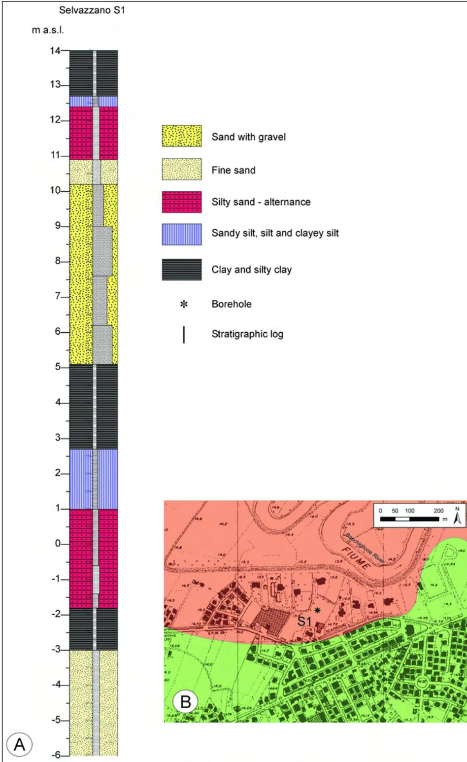
Fig. 8 - Stratigraphic log of S1 borehole at Selvazzano Dentro (A) and location map (B).
