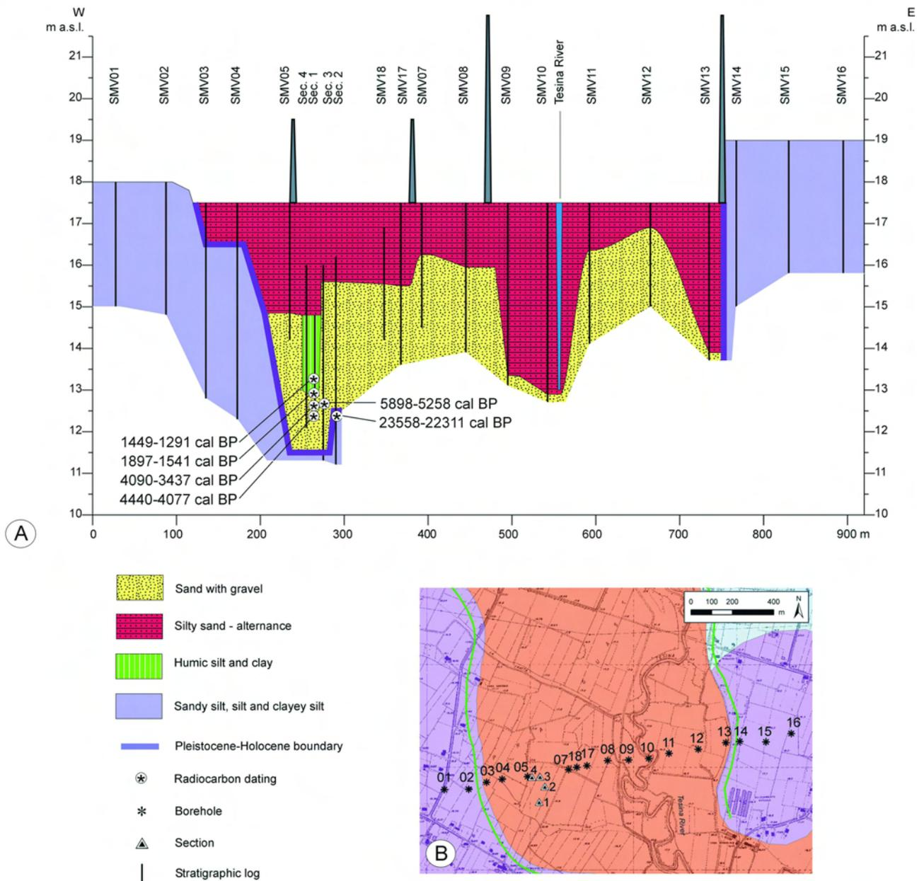
Fig. 7 – SM Veggiano cross section (A) and location map (B).
