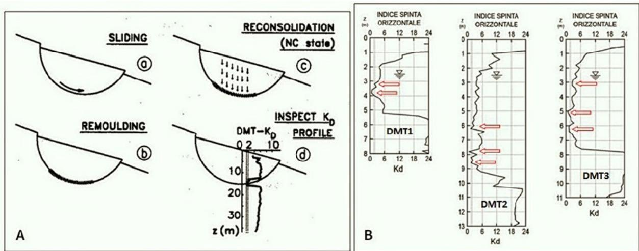
Fig. 3 - A) DMT-KD method for detecting slip surface in OC clay slopes from Totani et al., 1997 B) detecting failure surfaces by DMT in the Panicaglia site.
