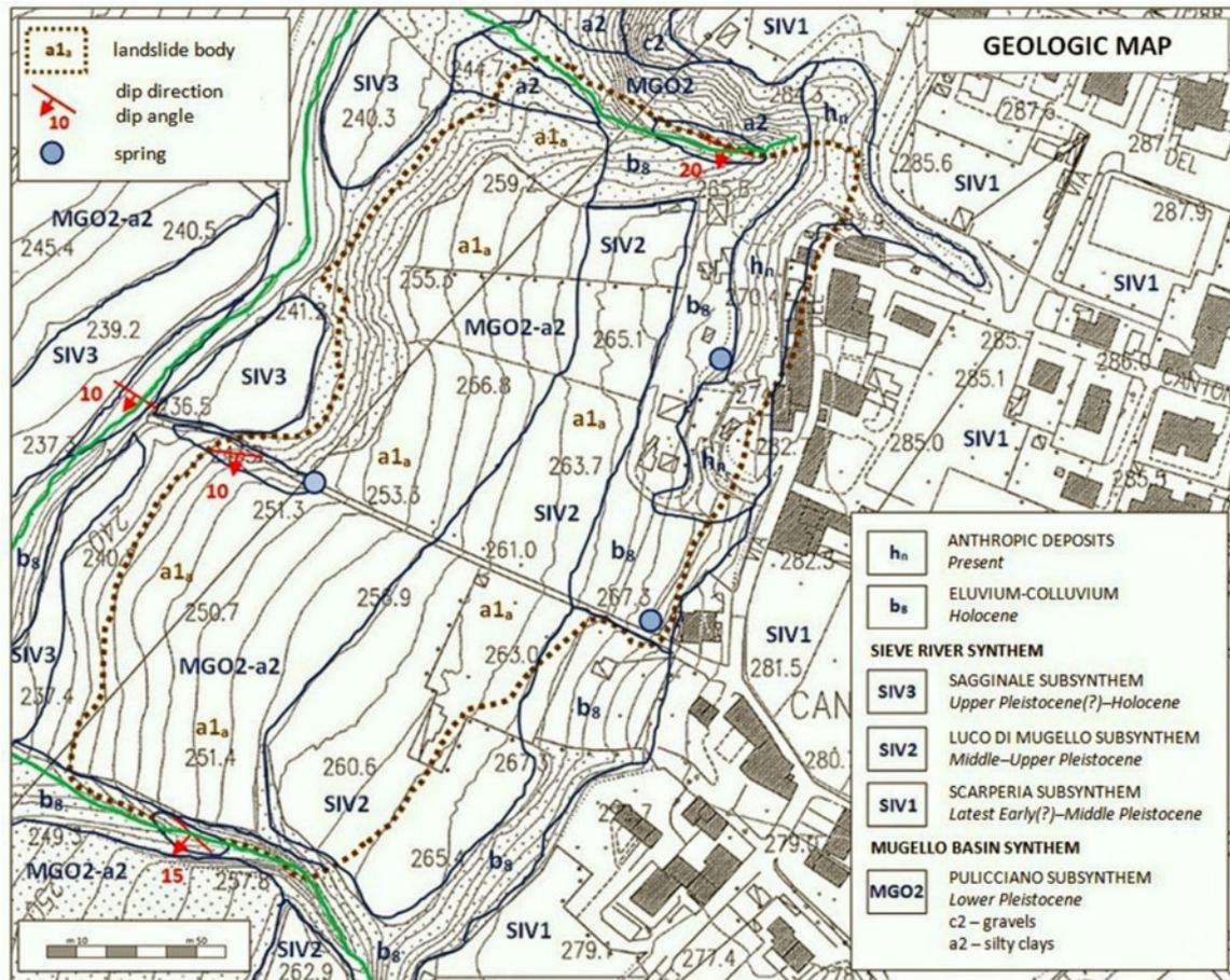
Fig. 1 - Panicaglia Landslide Geologic Map.
