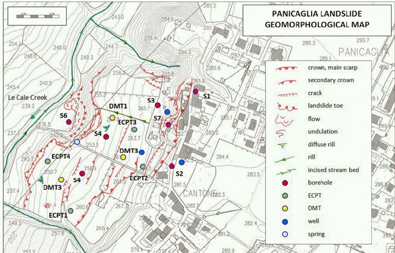
Fig. 2 - Panicaglia Landslide Geomorphological Map (topographic base map is Regione Toscana Technical Map – CTR, enhanced with conventional topographical survey).
