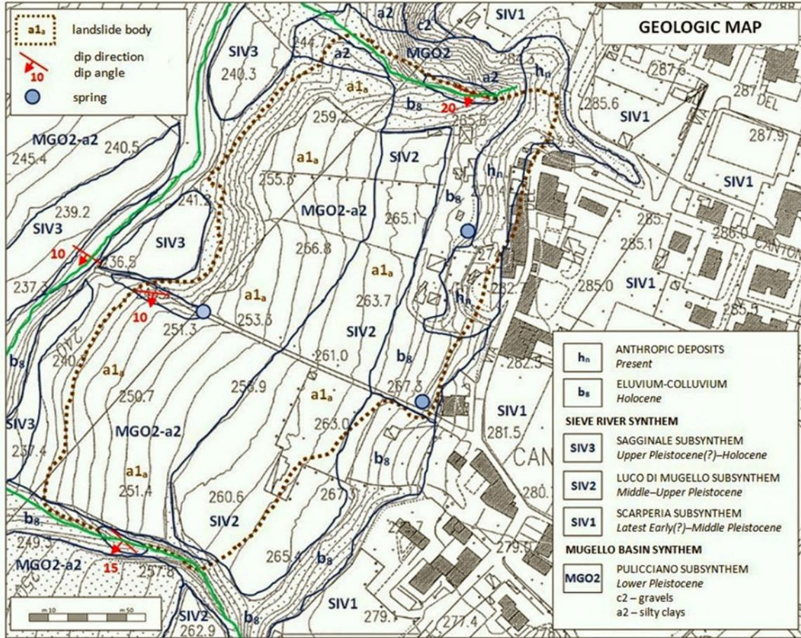
Fig. 1 - Panicaglia Landslide Geologic Map.
