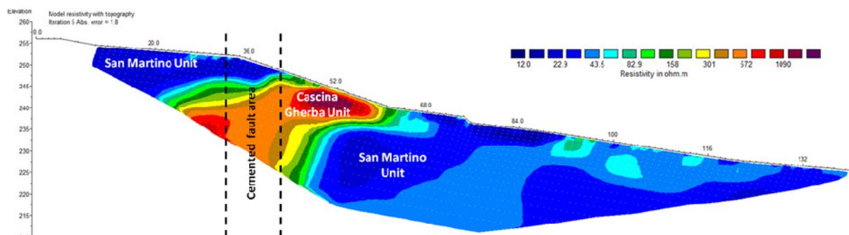
Fig. 4 - Resistivity distribution along the Cascina Volpiano geophysical survey line, with reported geological interpretation.
