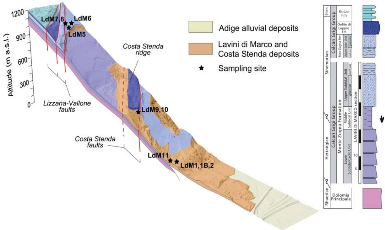
Fig. 4 - Schematic geological section of the Lavini di Marco and Costa Stenda rock avalanche deposits. Samples collected along the section are also shown (from Martin et al., 2014; Elsevier used with permission).
