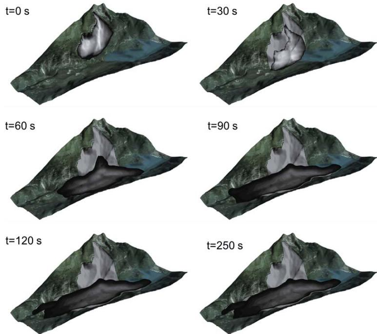
Fig. 14 - Time series of the run-out model for the Molveno rock-avalanche. The extent of the observed deposit is well reproduced (from von Wartburg et al., 2020).
