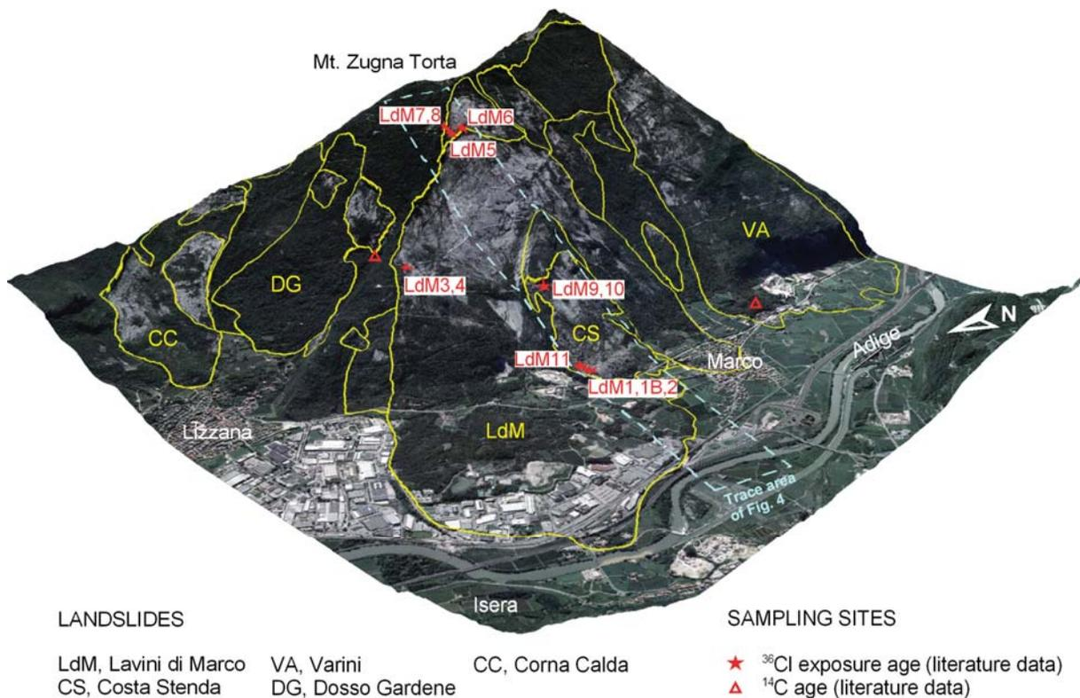
Fig. 2 - Landslide scarps and deposits along the western slope of Mt. Zugna Torta (from Martin et al. 2014; Elsevier used with permission). Stars mark the  $^{36}\text{Cl}$  dated samples for Lavini di Marco (LdM) and Costa Stenda (CS). Red triangles mark sites of  $^{14}\text{C}$ -dated samples (Orombelli & Sauro, 1988) (cf. Fig. 5).
