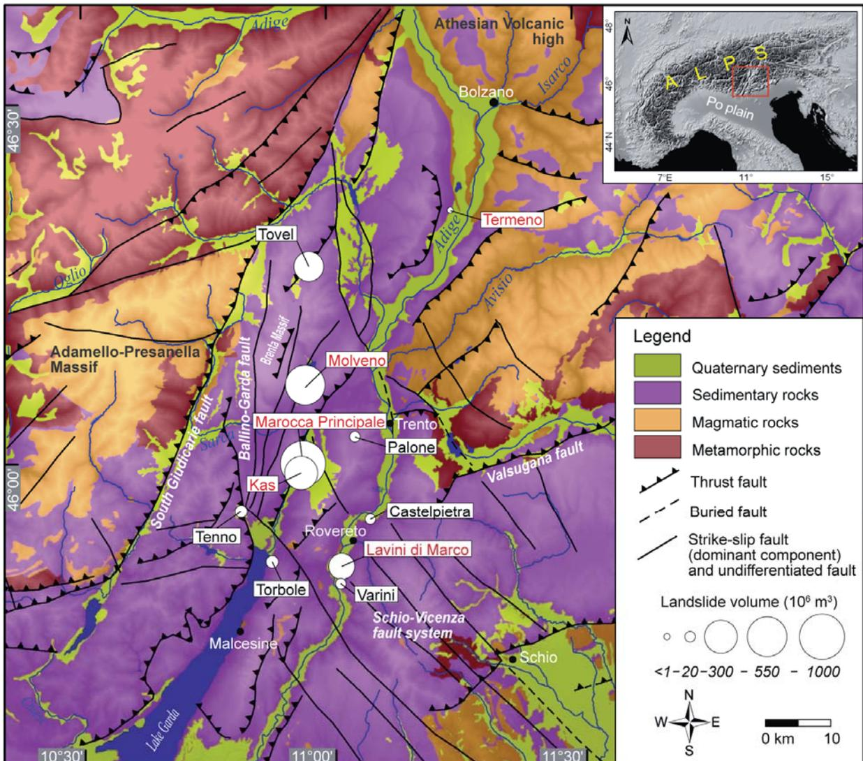
Fig. 1 - Simplified geological map of the Sarca and Adige Valleys (data from the Geological Survey of Trento, CARG project database). Circle size is proportional to landslide volume (modified from Ivy Ochs et al., 2017b; Elsevier used with permission). The Tovel deposits, with an estimated total volume of 300 Mm<sup>3</sup> (Oetheimer, 1989) and shown as a single circle, are due to multiple events. The names of the landslides studied in this work are in red.
