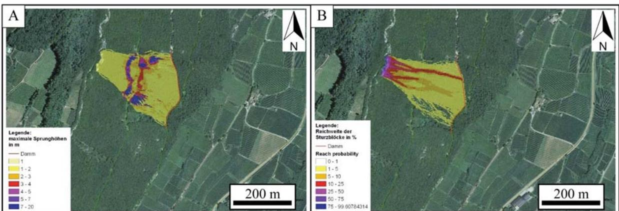
Fig. 8 - Simulation of failures with the planned dam. Left - jump height. Right: reach probability.
