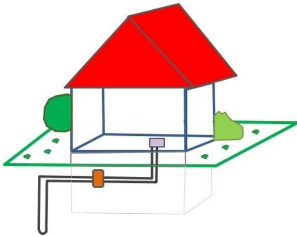
Fig. 2 - Closed-loop vertical system with downhole heat exchanger (DHE).
