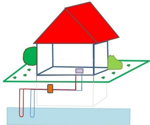
Fig. 3 - Open-loop system, with groundwater heat pump GWHP.
