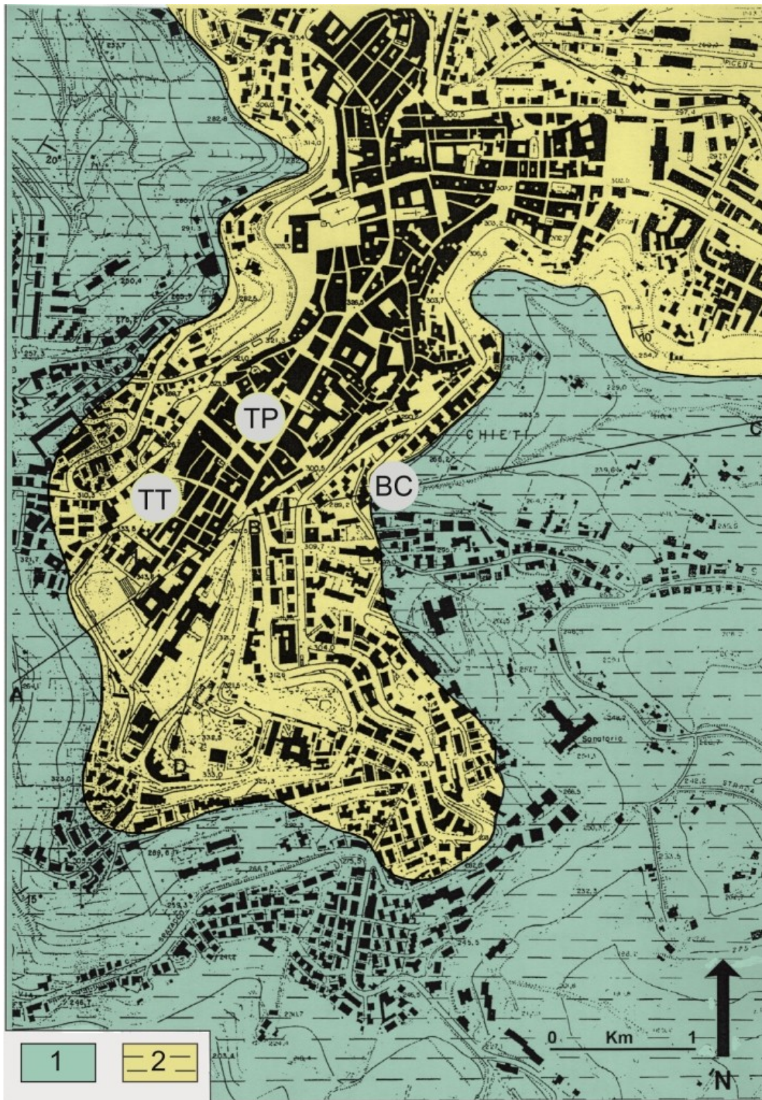
Fig. 2 - Simplified geo-lithological map: 1 - sand with lenses of conglomerate (U2 and U2 cgl in Fig. 3), gravel and lacustrine clays (U3 in Fig. 3), colluvial and anthropic sediments (U1 cl and U1 r in Fig. 3); 2 - clays (U1 in Fig. 3); TT - Roman Theatre area, TP - Roman Temples area, BC - Roman Baths and Cisterns area. A-B-C, D-B: trace of geological cross-section (Fig. 3).
