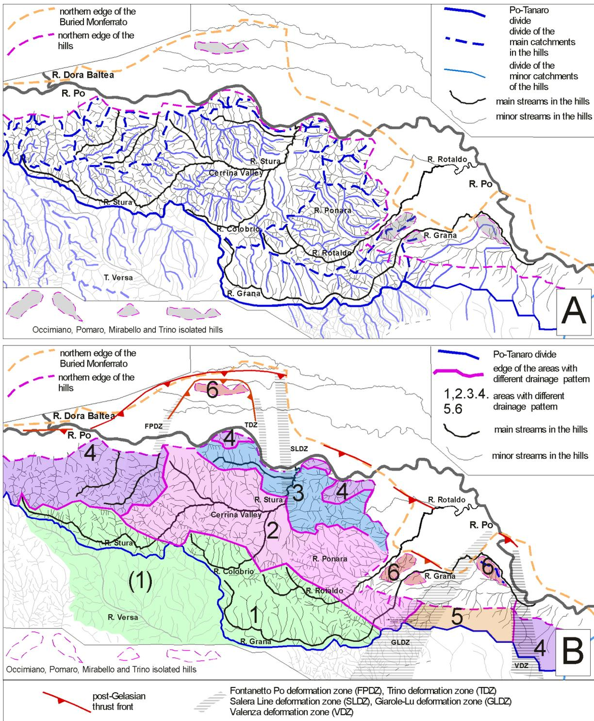
Fig. 5 - Drainage network and areas with a different drainage pattern in the Monferrato Hills and the Buried Monferrato. A: drainage network and catchment basins. B: areas with different drainage patterns.
