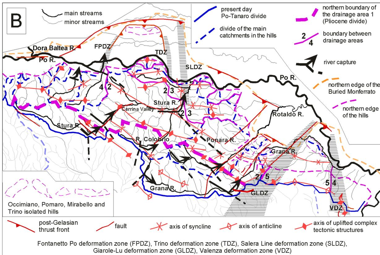
Fig. 6 - Asymmetry of the valleys and elbows of capture (6A) and relations between the drainage network and major tectonic features (6B).
