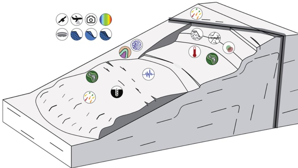
Fig. 1 - Structural features and controls (such as folds, fault zones, rock bridges, crown cracks, transverse cracks and ridges, and radial cracks) on landslides, with methods used to investigate them represented by icons. See Tab. 1 for legend of icons.
