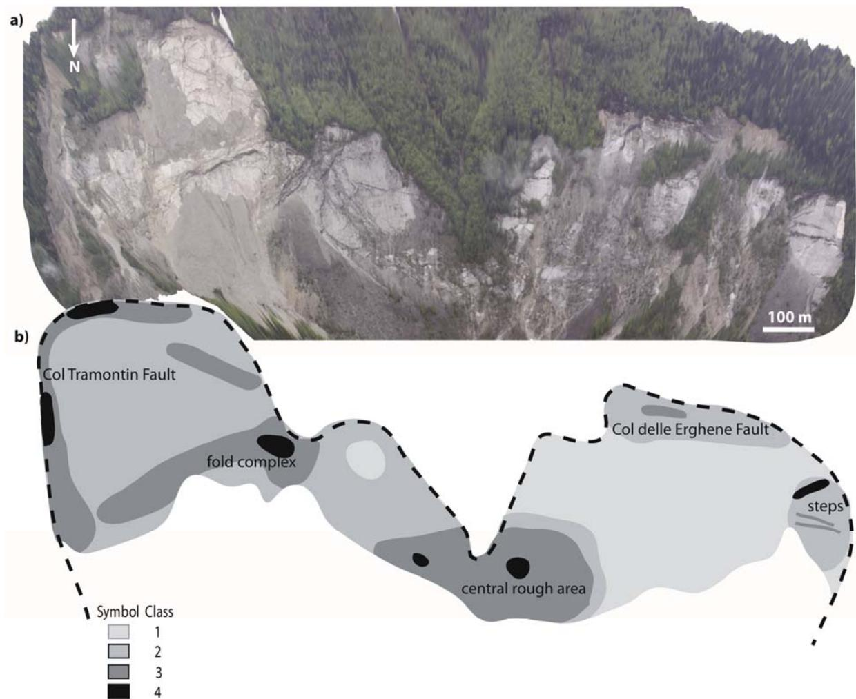
Fig. 3 - Roughness classes on the Vajont Landslide scar, based on block statistics. Class 1 represents areas that are largely planar and smooth, with roughness increasing to Class 4. Rougher areas are more likely to have caused dilation of the failure mass over asperities and/or rock bridge failure through asperities, with implications for movement behaviour. (Source: Wolter et al., 2014.)
