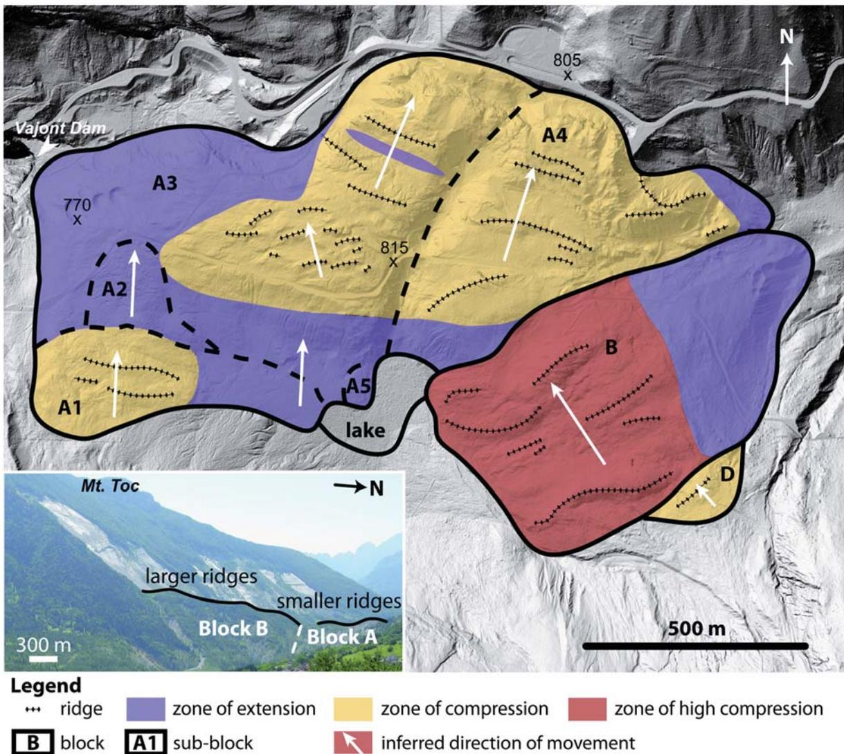
Fig. 4 - Morphostructural features of the Vajont Landslide deposits, showing zones of extension and compression, as well as blocks within the deposit. (Source: Wolter et al., 2015.)
