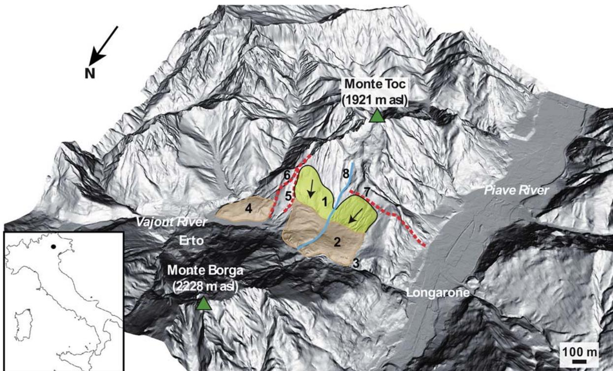
Fig. 2 - Location and context of the Vajont Landslide. 1 - Vajont Landslide failure scar, 2 - Vajont Landslide deposit, 3 - Vajont Dam, 4 - Pineda Landslide deposit (prehistoric failure), 5 - Col Tramontin Fault, 6 - Croda Bianca Fault, 7 - Col delle Erghene Fault, 8 - Massalezza Stream. (Modified after: Wolter et al., 2014.)
